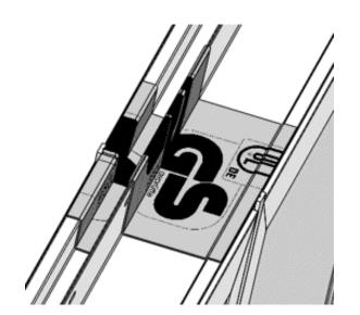
Apply self-adhesive flashing tape over the top side of mull gap and over nail fin at the head and sill.
