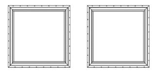
Lay the units down on a drop cloth or cardboard in the order they are to be mulled with exterior side down.
