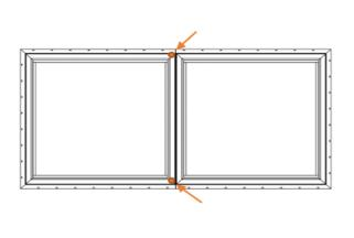
Place the windows together and add a small amount of sealant at the top and bottom of the mull channel before driving in the mulls.
