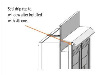
Install drip cap over the nail fin the full length of mulled units at the head.
