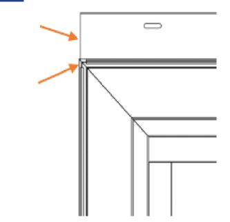
Cut a notch in the accessory channels in the head and sill to allow for mull key to set flush.
