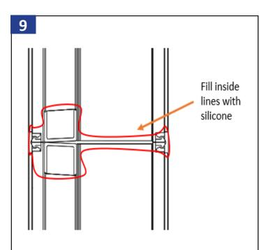
Seal both ends of the mull gap with silicone the entire width of the frame at the head and sill.
