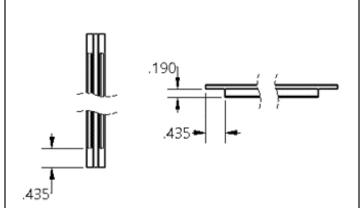
Cut the C-mull keys to the length of the unit (width or height) to be mulled.
