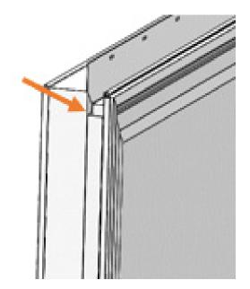
Install the j-channel filler into j-channel slot on the side to be mulled of the exterior of each window. Cut the filler short of head and sill j-channel slot so as not to obstructed the channel.
