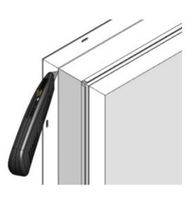
Using a utility knife score and remove the nailing fin from each unit where the mull will connect them. Make sure to cut the head and sill nail fins back flush with frame.
